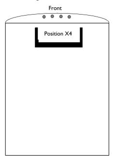
3. Mount the memory module by sliding it into the X4 socket at an angle of 45 degrees. Once the module is fully inserted, press it downwards towards the PCB, until the socket locks the module into place.
